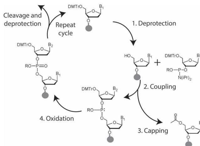
**FIGURE 6.3** Automated organic synthesis of DNA oligonucleotide on solid support with the phosphoramidite method [50].
