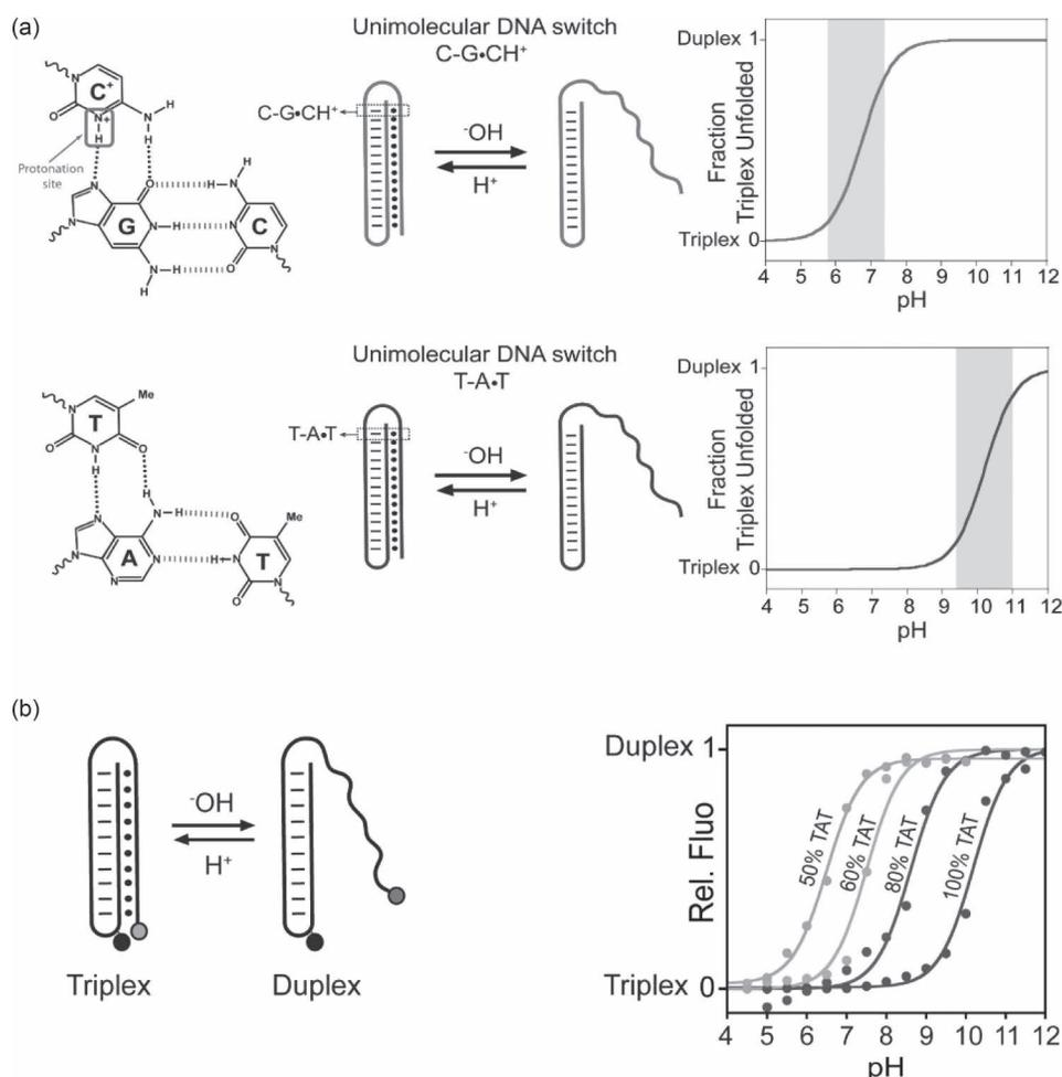
**FIGURE 6.13** (a) Parallel triplex DNA structures were used to create pH-sensitive DNA switches to monitor pH variations (nano pH meter). (b) DNA pH meter has pH sensitivity that can be modulated by changing their DNA sequence with parallel triplex TAT or CGC. (Adapted with permission from Ref. [75]. Copyright 2014 American Chemical Society.)
