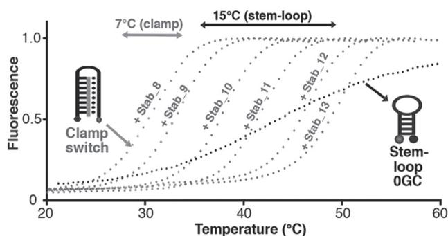
**FIGURE 6.12** DNA clamp switch structures can be used to build nanothermometers with increased sensitivity to probe smaller temperature variations with high precision. (Adapted with permission from Ref. [61]. Copyright 2016 American Chemical Society.)
