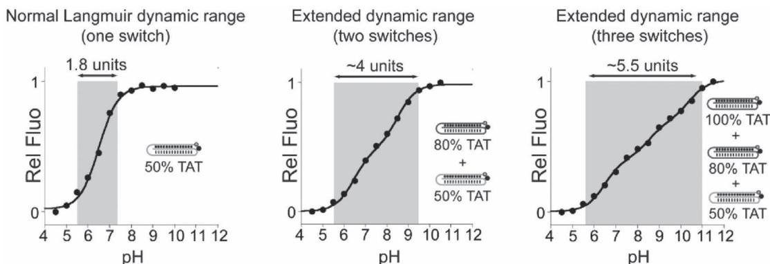
**FIGURE 6.14** Combining DNA pH meter of different pH sensitivity can yield extended pH monitoring capacity. (Adapted with permission from Ref. [75]. Copyright 2014 American Chemical Society.)
