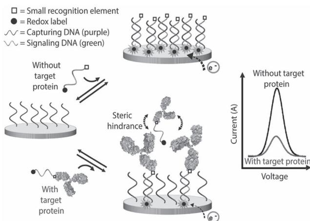
**FIGURE 6.16** Steric hindrance was exploited to engineer a DNA switch for the detection of large biomarkers using gold electrodes. (Adapted with permission from Ref. [114]. Copyright 2015 American Chemical Society.)
