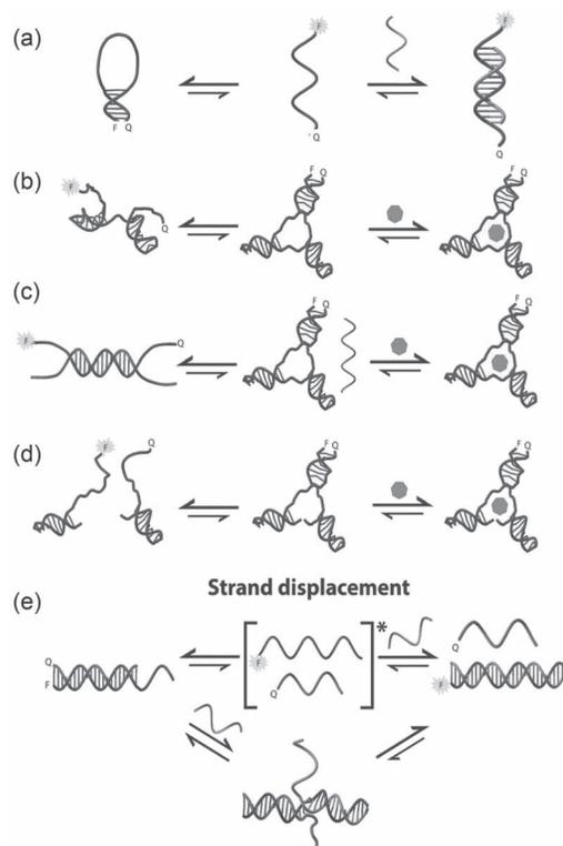
**FIGURE 6.6** Engineering strategies to introduce a switching mechanism in DNA recognition elements. F: fluorophore; Q: quencher. (Adapted from Ref. [12] with permission from The Royal Society of Chemistry.)
