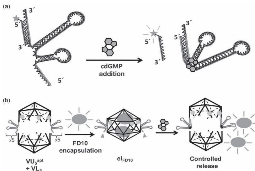
**FIGURE 6.22** (a) A DNA aptamer was adapted into a DNA switch that undergoes conformational change upon binding to its input molecule c-di-GMP. (b) This DNA switch was inserted on a DNA cage whose opening, and drug cargo release, is triggered by activation of the DNA switch in the presence of c-di-GMP. (Reprinted with permission from Ref. [157]. Copyright 2013 John Wiley and Sons.)
