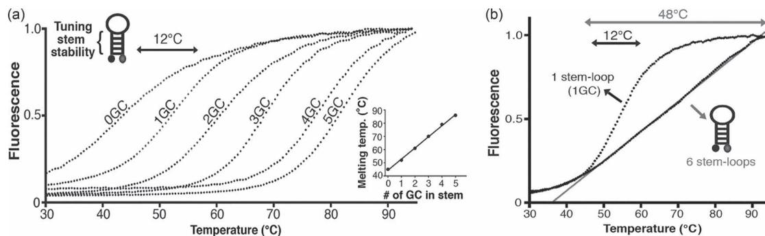
**FIGURE 6.10** (a) Molecular beacons can be thermodynamically engineered into DNA nanothermometer tools with various temperature sensitivity. (b) Combining multiple DNA thermometers with different  $K_S$  results in an extended linear range to monitor extended temperature variations. (Adapted with permission from Ref. [61]. Copyright 2016 American Chemical Society.)
